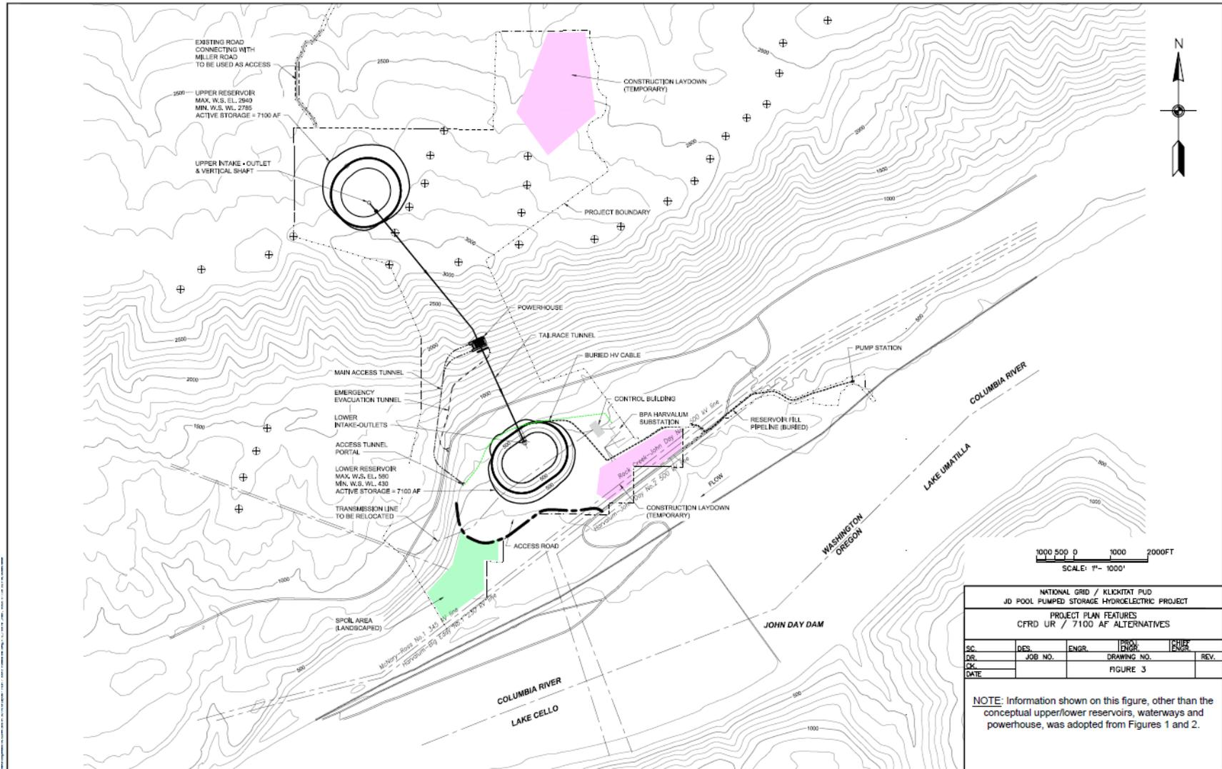
Figure 1.5-1: Goldendale Energy Storage Project General Arrangement—Alternative 1—Plan
